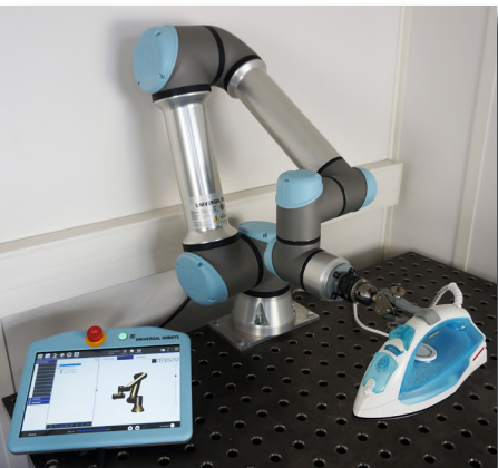
> Endurance test on irons according to standard: IEC 60311 (Performance measurement method)
